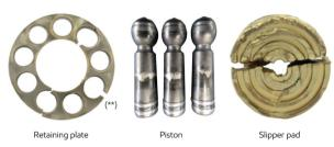
(\*\*) Retaining plate failure caused by slipper pad damage.
